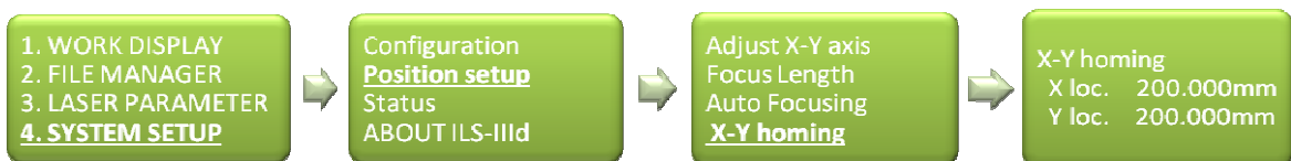
Obr. 27 Nabídka SYSTEM SETUP- Position setup – X-Y homing
