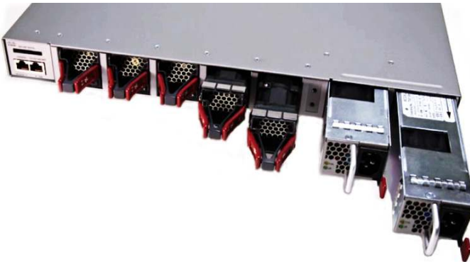
Figure 7. Redundant Fan and Power Supply
