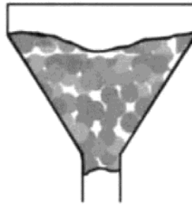
Figure 3-5 Feed hopper bridging
