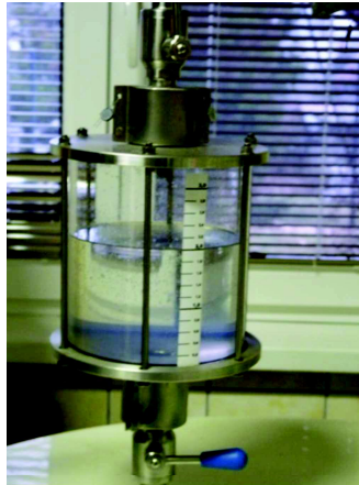
Drips and drops collecting container attached to collecting tank, Figure 2
