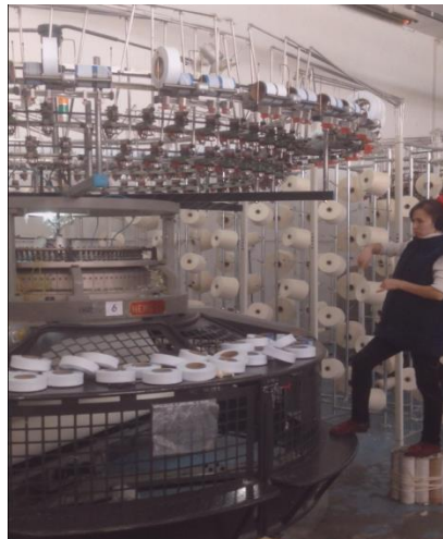
Figure 32: Yarn feeding process by operator
