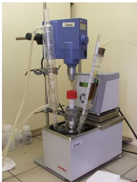
Fig. 4: Assembly used for iron oxide NPs synthesis.
