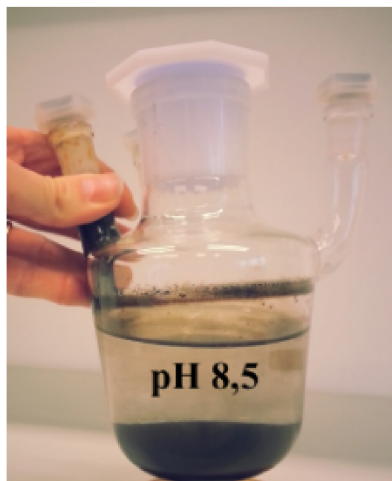
Fig. 5: Sedimentation of MCPs at the bottom of the flask after synthesis.
