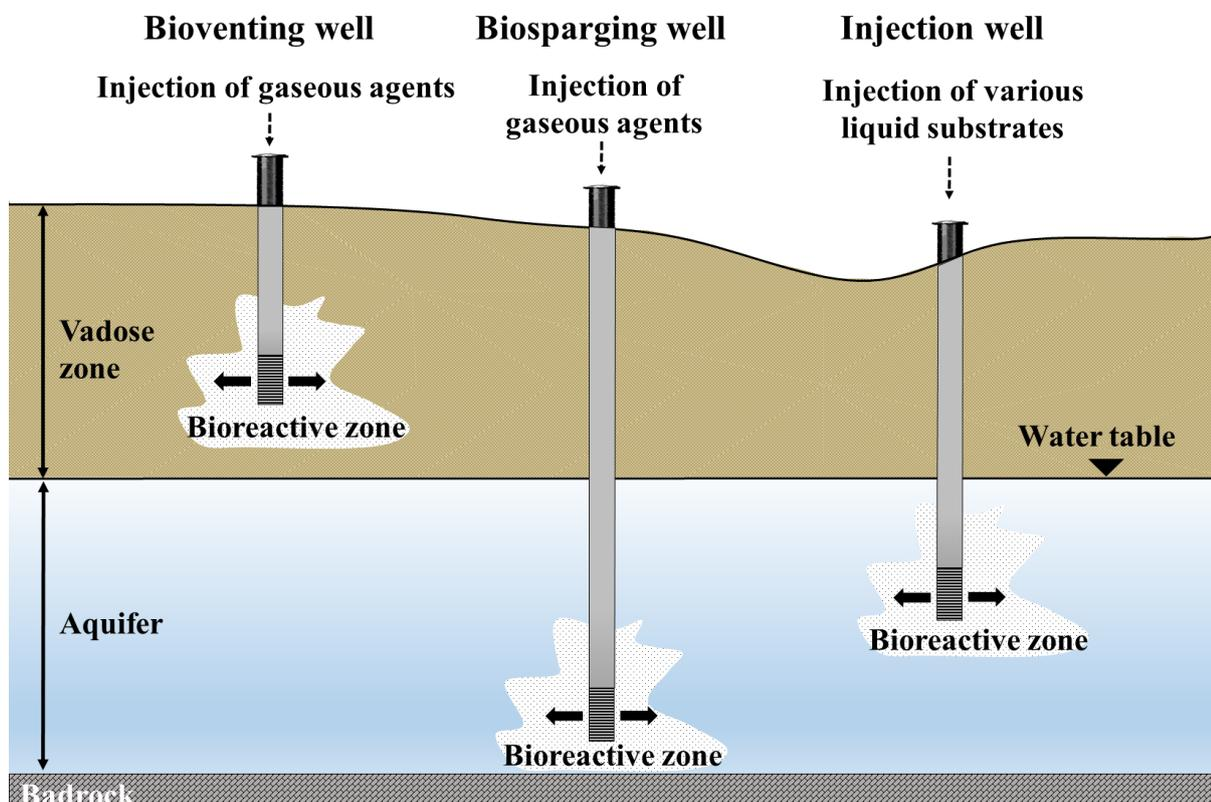
*Fig. 1.7 Wells for biostimulation of microbial degradation of CEs in a subsurface environment<sup>4</sup>*
