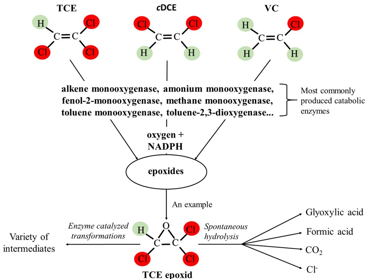
*Fig. 1.5 Cometabolic oxidation of CEs*
