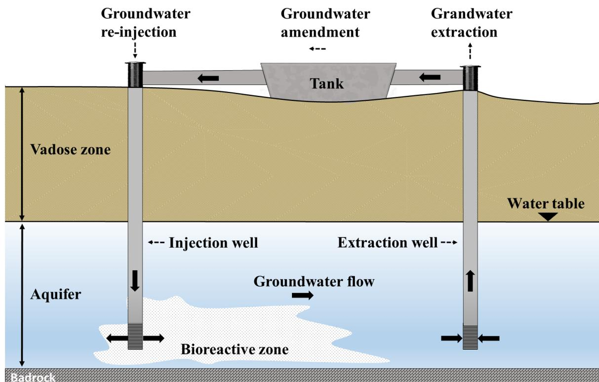
*Fig. 1.8 Closed loop system<sup>5</sup>*
