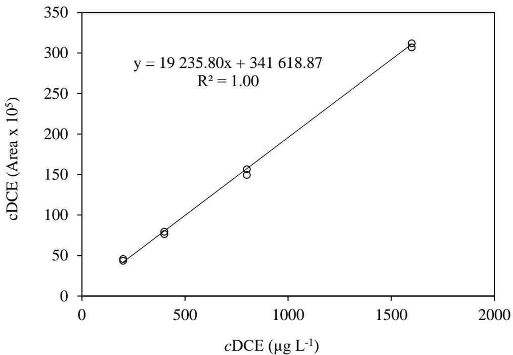
Fig. 3.1 Calibration curve of cDCE (concentration range from  $200 \mu\text{g L}^{-1}$  to  $1600 \mu\text{g L}^{-1}$ )
