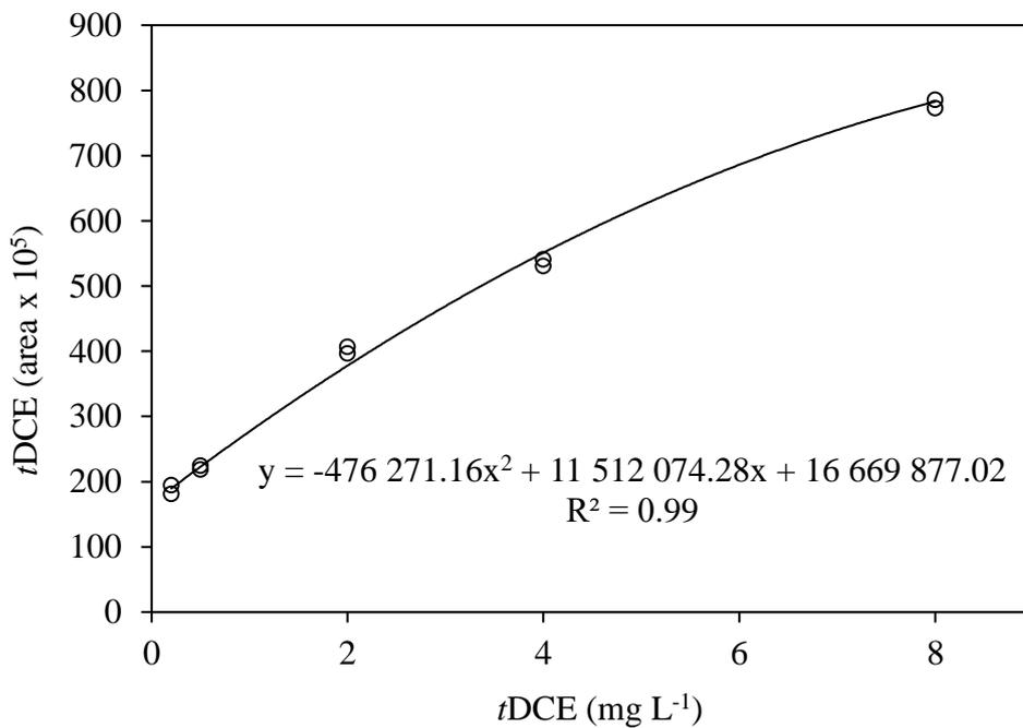
Fig. 3.2 Calibration curve of tDCE (concentration range from  $200 \mu\text{g L}^{-1}$  to  $8000 \mu\text{g L}^{-1}$ )
