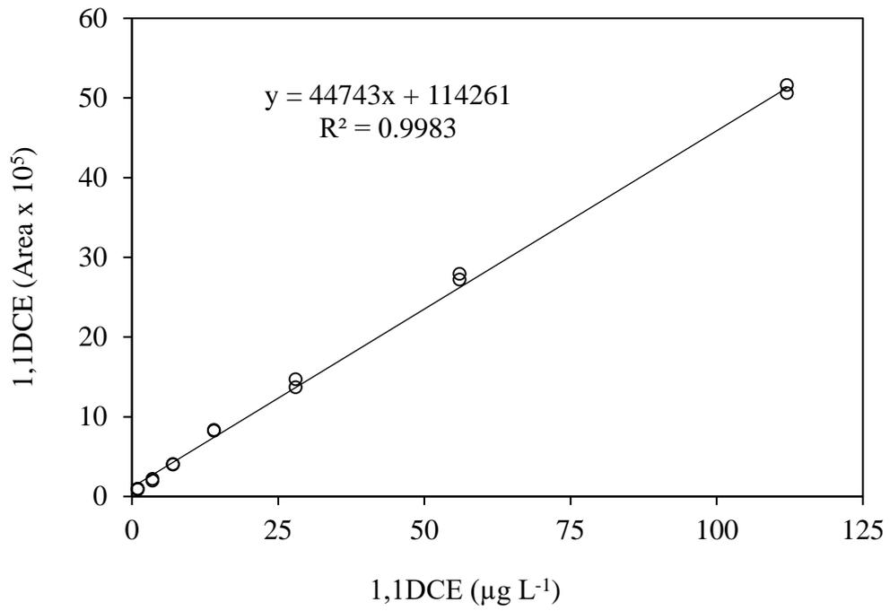
Fig. 3.3 Calibration curve of 1,1DCE (concentration range from  $1 \mu\text{g L}^{-1}$  to  $112 \mu\text{g L}^{-1}$ )
