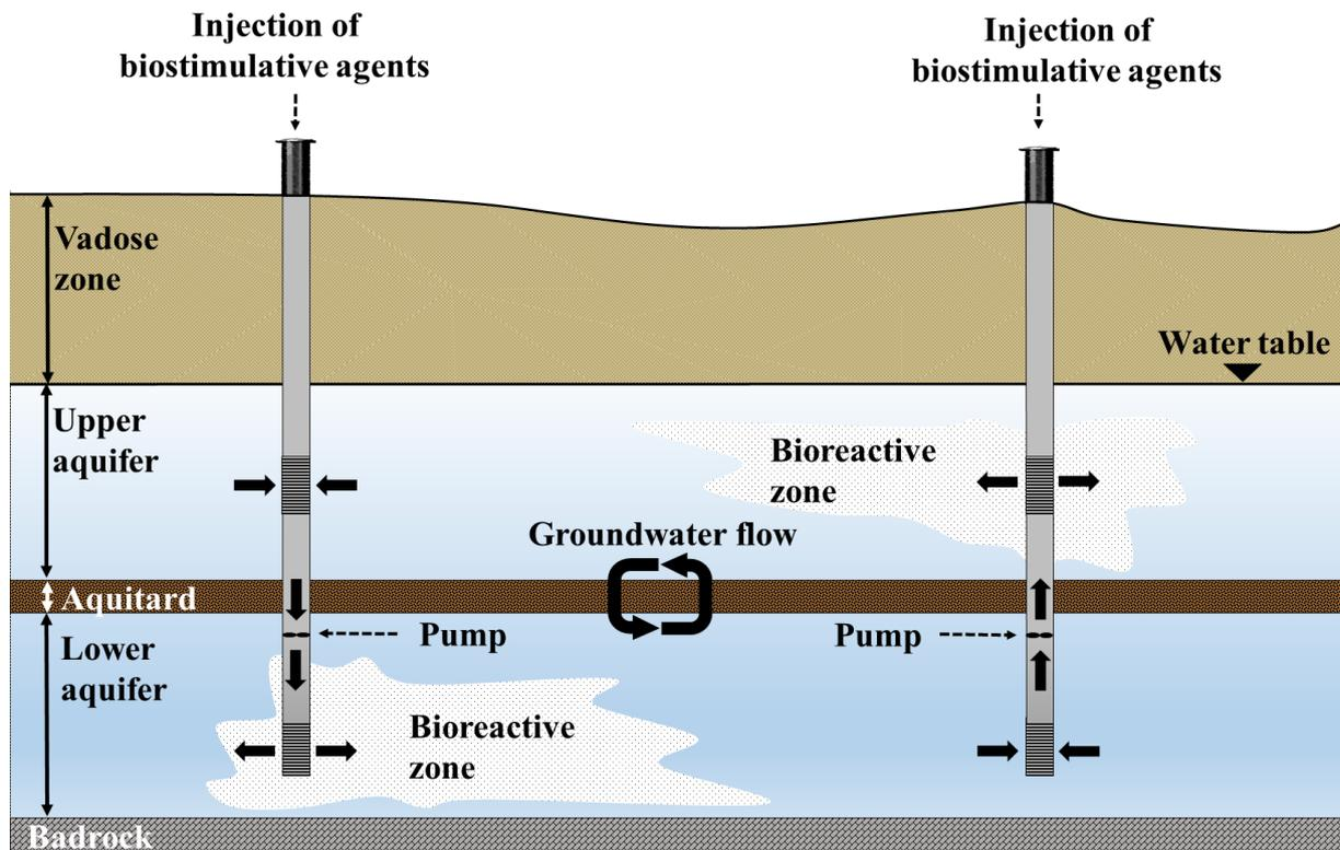
Fig. 1.9 System employing two recirculation wells<sup>6</sup>
