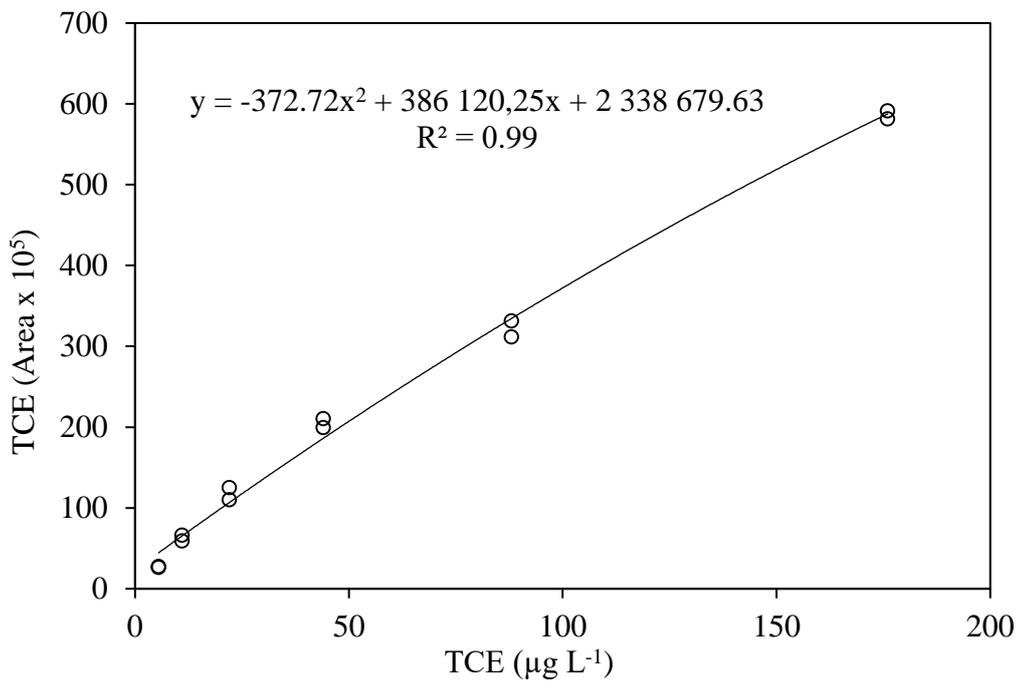
Fig. 3.4 Calibration curve of TCE (concentration range from  $5.5 \mu\text{g L}^{-1}$  to  $176 \mu\text{g L}^{-1}$ )
