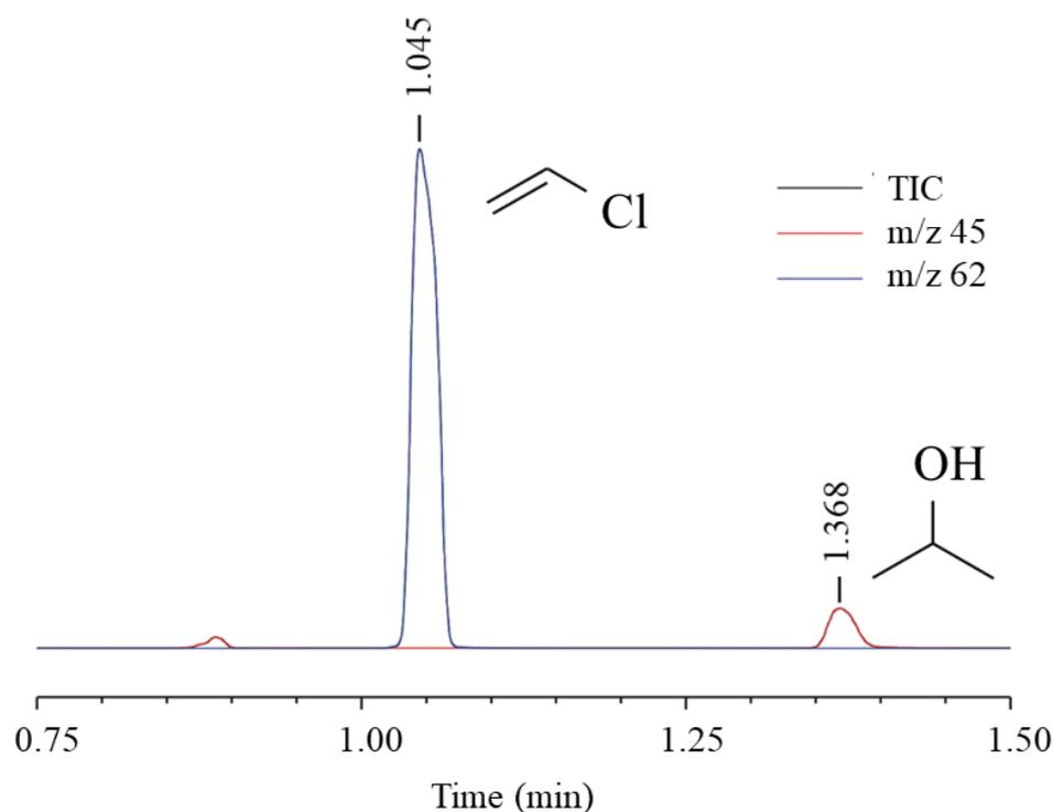
Fig. 3.5 Characteristic ions and retention times for VC and IPA on a portion of the typical chromatogram<sup>7</sup>
