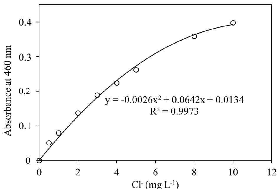
*Fig. 3.6 Calibration curve for determination of inorganic  $\text{Cl}^-$  in degradation samples containing chloroethenes<sup>8</sup>*
