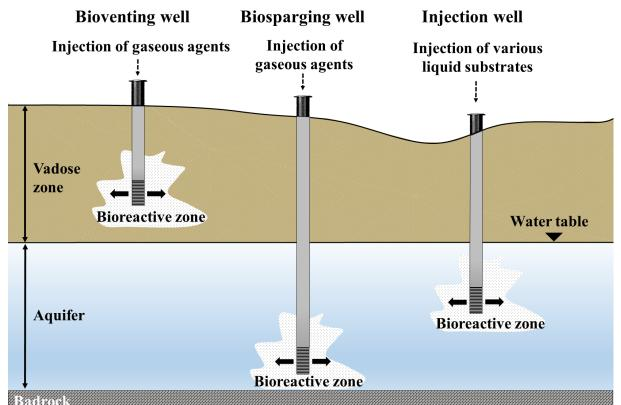
Fig. 1.7 Wells for biostimulation of microbial degradation of CEs in a subsurface environment<sup>4</sup>
