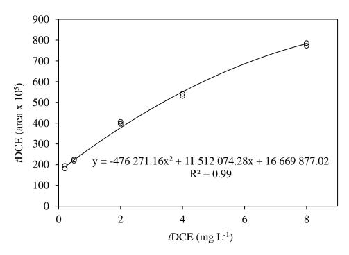
Fig. 3.2 Calibration curve of tDCE (concentration range from  $200 \ \mu g \ L^{-1}$  to  $8000 \ \mu g \ L^{-1}$ )
