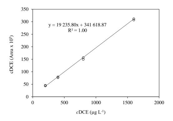
Fig. 3.1 Calibration curve of cDCE (concentration range from  $200 \ \mu g \ L^{-1}$  to  $1600 \ \mu g \ L^{-1}$ )
