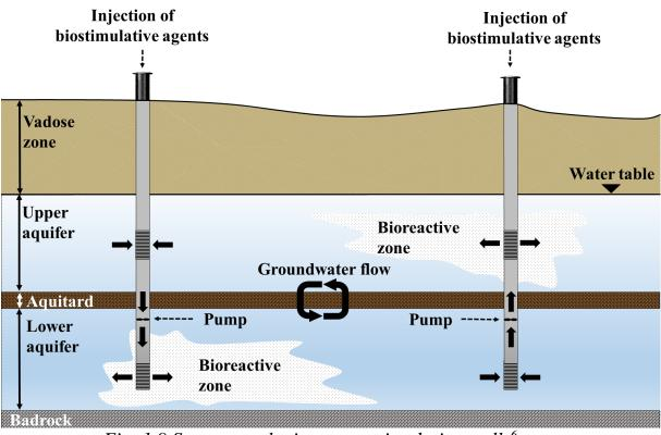
Fig. 1.9 System employing two recirculation wells<sup>6</sup>
