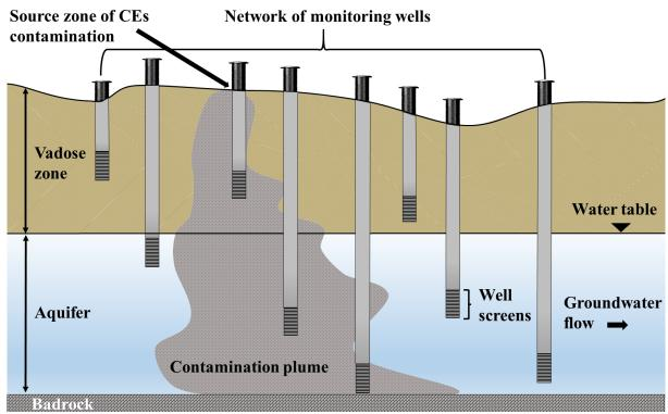
Fig. 1.6 Schematic of a site monitoring using a network of monitoring wells
