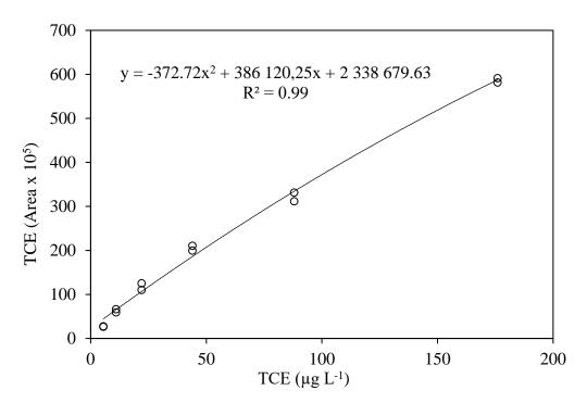
Fig. 3.4 Calibration curve of TCE (concentration range from  $5.5 \ \mu g \ L^{-1}$  to  $176 \ \mu g \ L^{-1}$ )
