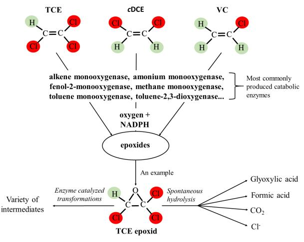
Fig. 1.5 Cometabolic oxidation of CEs
