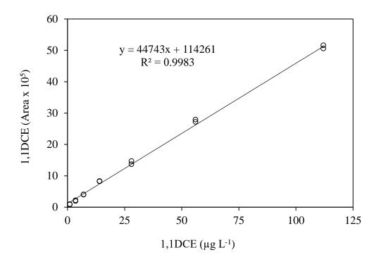
Fig. 3.3 Calibration curve of 1,1DCE (concentration range from  $1 \ \mu g \ L^{-1}$  to 112  $\mu g \ L^{-1}$ )
