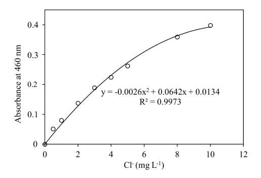
*Fig. 3.6 Calibration curve for determination of inorganic Clin degradation samples containing chloroethenes*<sup>8</sup>
