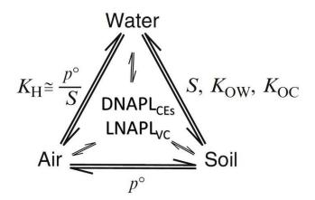
*Fig. 1.2 Major phases occurring in the subsurface and the properties of CEs that govern the partitioning between these phases*<sup>1</sup>
