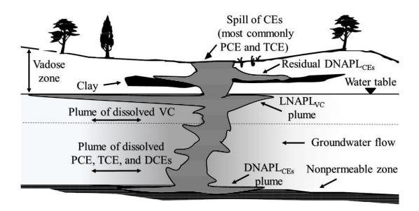
Fig. 1.3 Likely transport of CEs in the subsurface<sup>3</sup>
