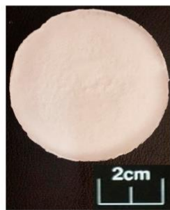
Figure 4. Photographic appearance of the PLA-PVA porous bioscaffold.
