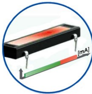
Obrázek 25 PSD – Position Sensitive Devector [14]
