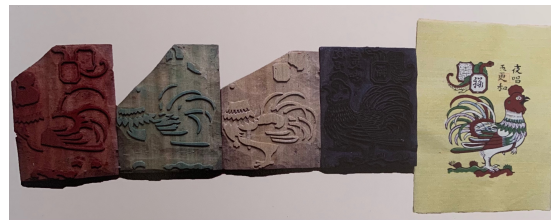
Fig. 15 Woodblock prints are used to print each color layer of Dong Ho folk paintings.
