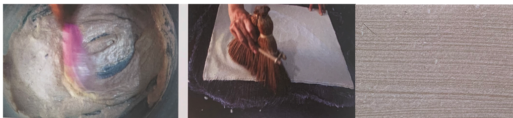
Fig. 21 Process of mixing scallop powder with glutinous rice and applying it on the surface of Do paper
