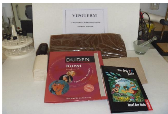
Fig. 3. Thermoplastic collagen adhesive used for gluing of book hard covers
