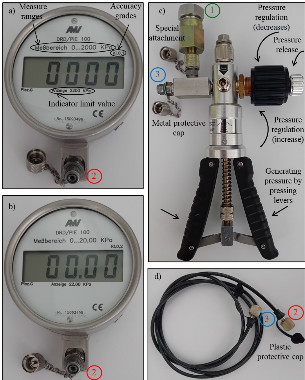
Figure 48 Used calibration device in an unconnected state. a) Indicator with a range of (0-2000) kPa, b) Indicator with a range of (0 – 20) kPa, c) View of the main part, i.e., the hand pump, which contains the entry for pressure sensor 1, d) Air hose connecting the indicator (input/output 2) and hand pump (input/output 3)
