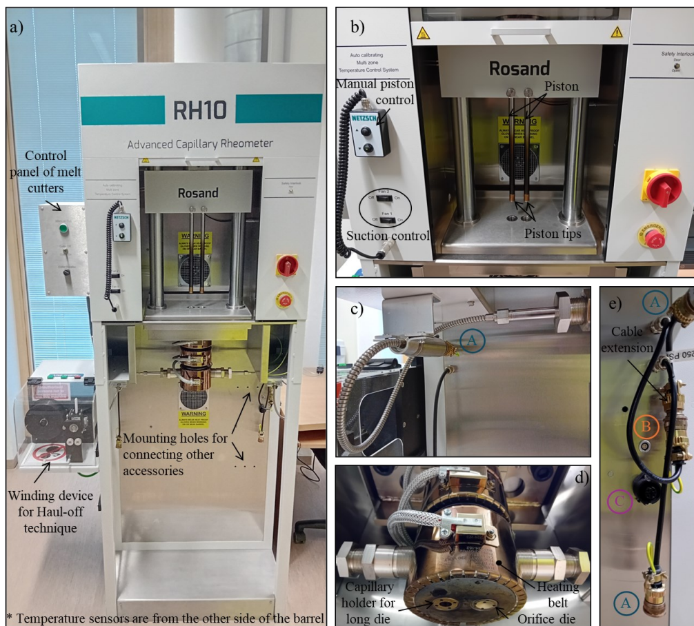
Figure 43 Rosand RH10 used in the experiment, a) general view including its accessories, b) view of the moving part, c) attachment of the pressure transducer and its connection via connector A (of which there are a total of 4 on the device), d) Bottom view of the heated barrel, e) Other connection options via connectors: B is for connecting the temperature sensor and C is for the heating belt
