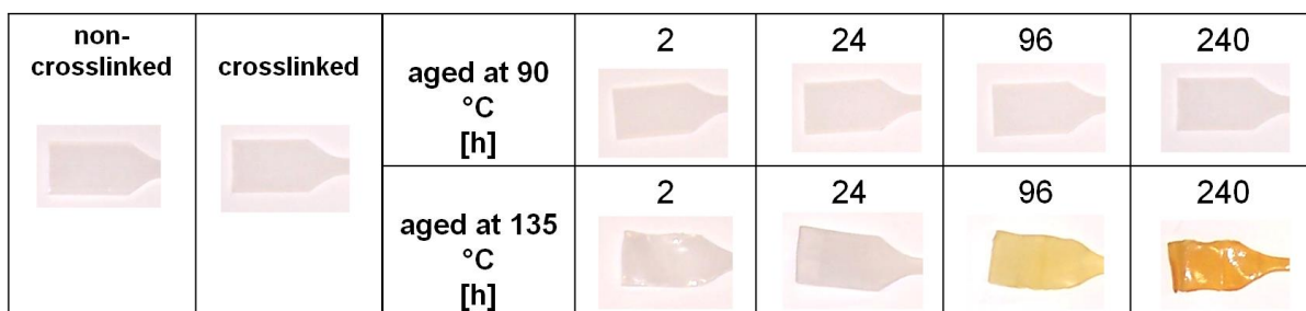
Fig. 6.4: Aged samples of Visico (0% Amb). Color changes start after 24 hours of ageing at 135 °C.
