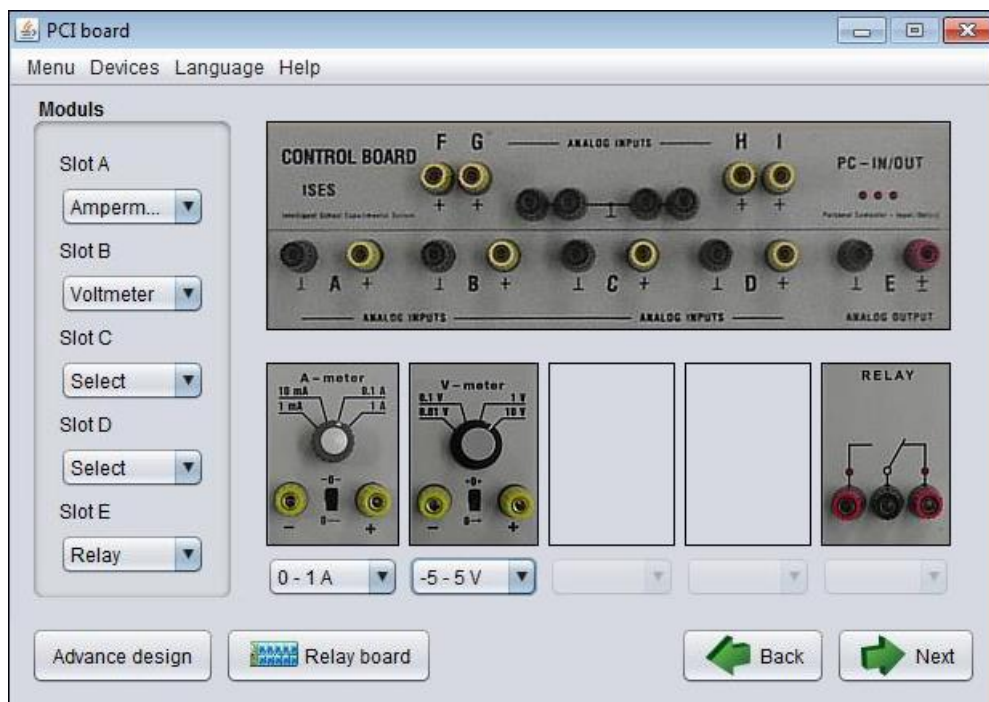
Figure 17 Modules selection window of the RL basic level that provides the intuitive setup for the ISES control board slots
