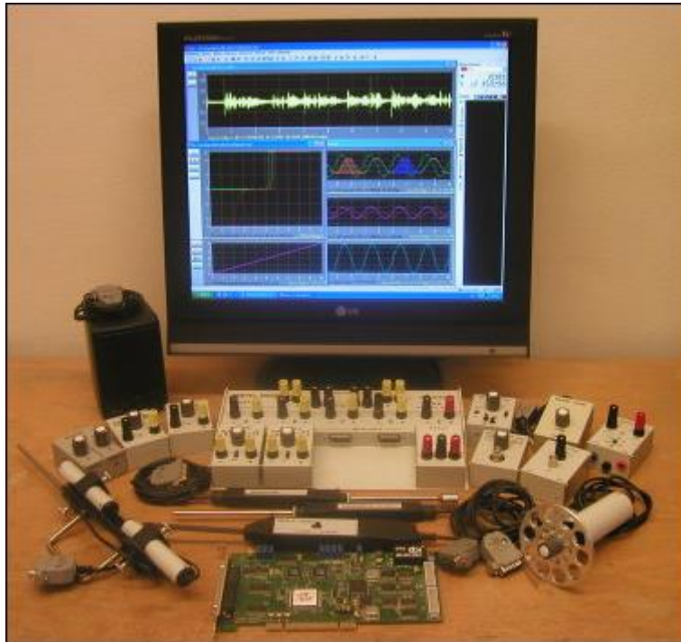
Figure 2 ISES physical hardware and software components; the PCI ADDA interface card, the set of meters, sensors and device
