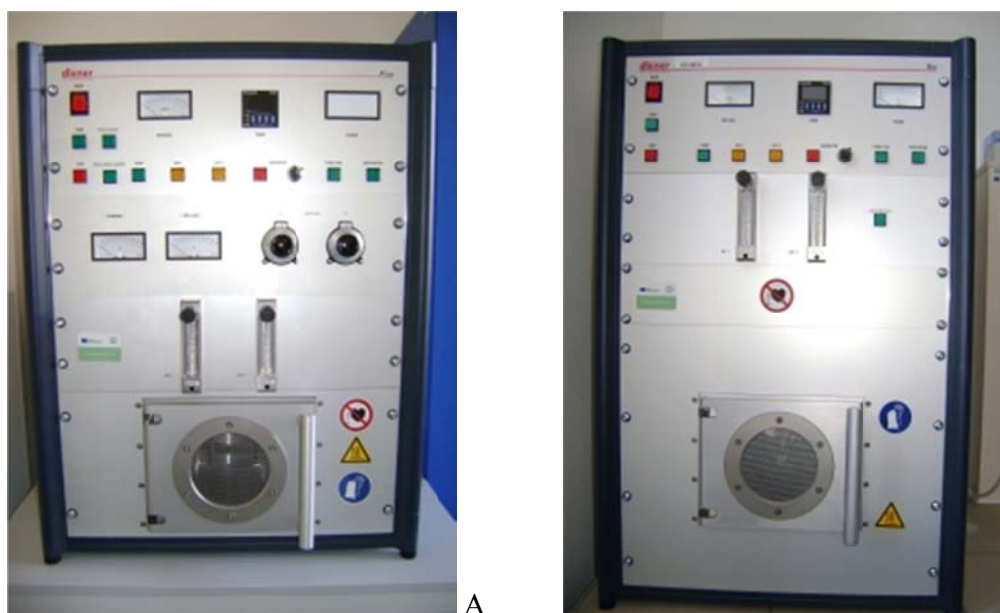
Fig. 1.: Plasma reactor. A - microwave frequency (2.45 GHz) and B - high frequency (40 kHz)
