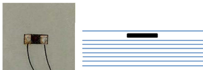
Fig. 2 a) An example of the test specimen which consist of MWCNT/TPU layer (black) laminated into epoxy/glass fiber composite with attached Cu electrodes. Part b) Schematic illustration of epoxy/glass fiber composite (8 layers glass fiber unidirectional) with MWCNT/TPU strain sensing layer (black stripe) used for bending tests.
