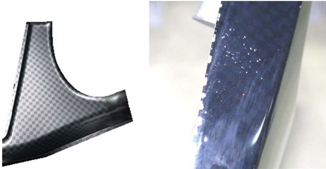
Figure 2 Dark color IMD foil with printed pattern after preforming (left) and after back-injection molding and following grinding of upper layers (right)
