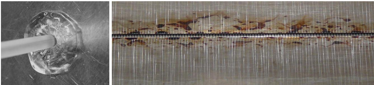
Fig. 7: Die drool phenomenon occurring during extrusion of HDPE melt through a single hole [87] (left) and during melt blowing of PP via multi hole MB die under processing conditions provided in [Paper IV] (right)
