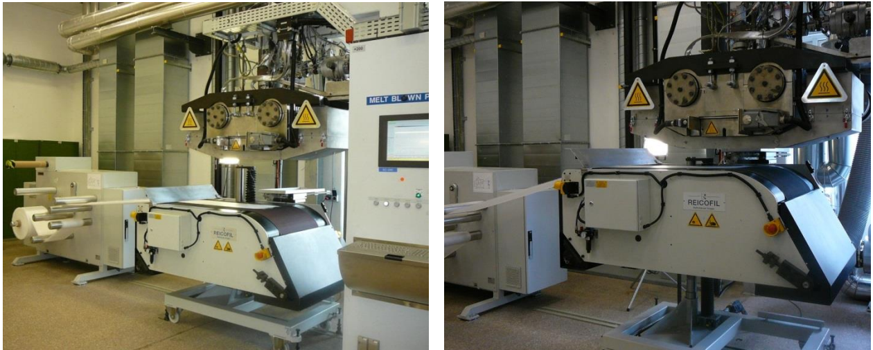
Fig. 25: MB pilot line for two different processing conditions: (left) DCD = 500 cm, (right) DCD = 200 cm
