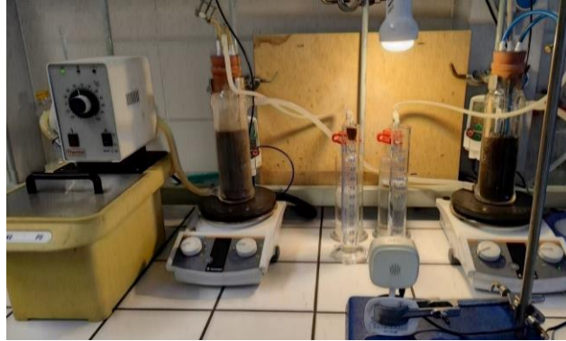
Figure 5.1. Experimental setup utilised for the anaerobic digestion
