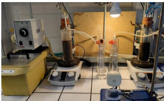
Figure 8.1. Experimental setup utilised for the anaerobic digestion
