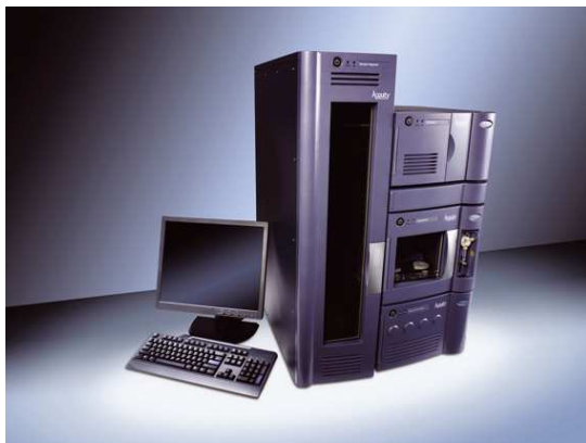
Obr. 33. Kapalinový chromatograf Acquity UPLC [46]
