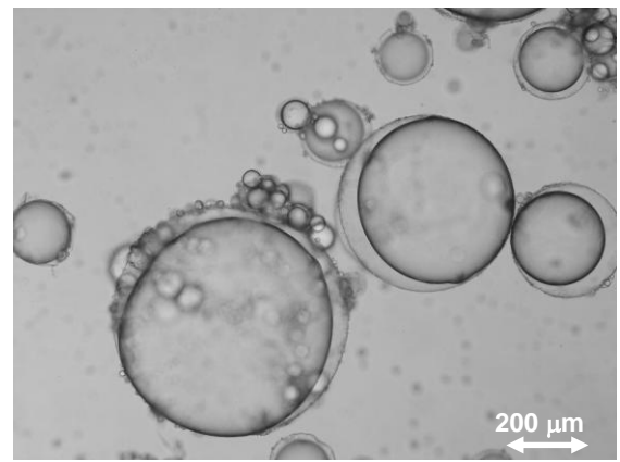
Figure 63: Optical micrographs of PVA 6-98/BCAR microcapsules after 48 hours release test in phosphate buffer (pH=7.4). Experiment J
