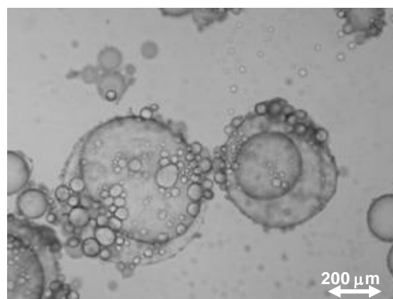
Figure 82: Optical micrographs of PVA 6-98/BCAR/LA 15 wt. % microcapsules after 6 hours in hydrochloride acid solution at 100 °C. Experiment L
