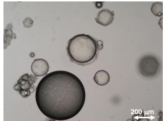
Figure 61: Optical micrographs of PVA 6-98/BCAR microcapsules after 48 hours release test in distilled water. Experiment F
