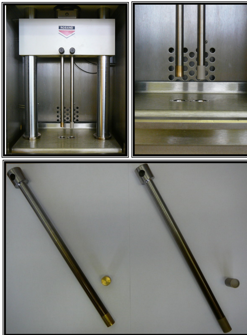
Fig. 16. Comparison between the PEEK (grey color piston tip) and copper piston tips for the capillary rheometer
