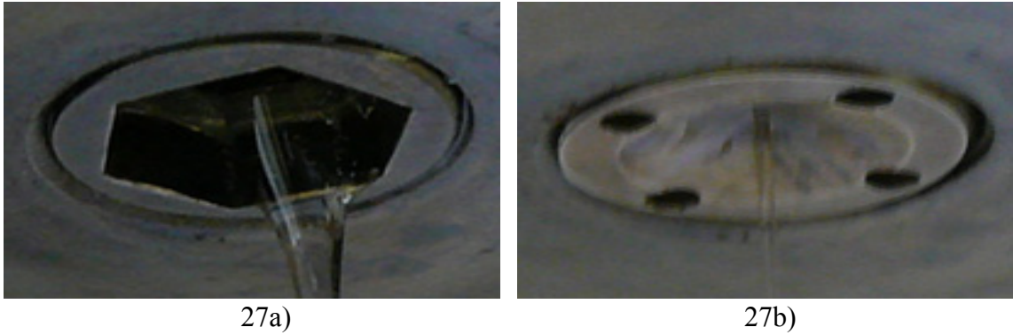
Fig. 27. Orifice downstream region during melt extrusion; 27a) Old orifice die design 27b) New design orifice die design
