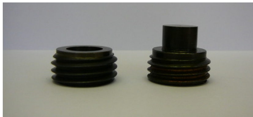
Fig. 24. Photo of new (left [35]) and old (right) orifice die design
