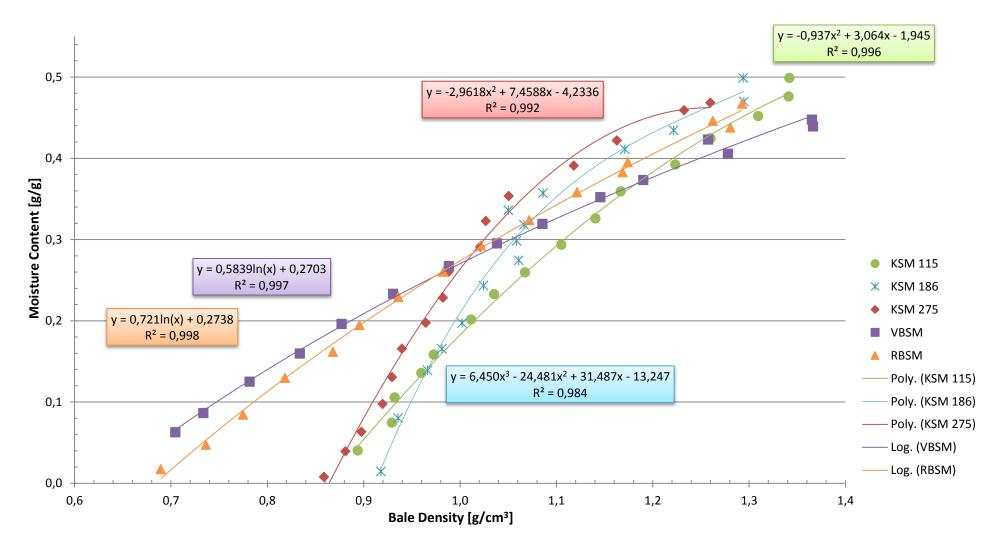
Figure 48. Moisture/density dependence of kraft & board sheet model.
