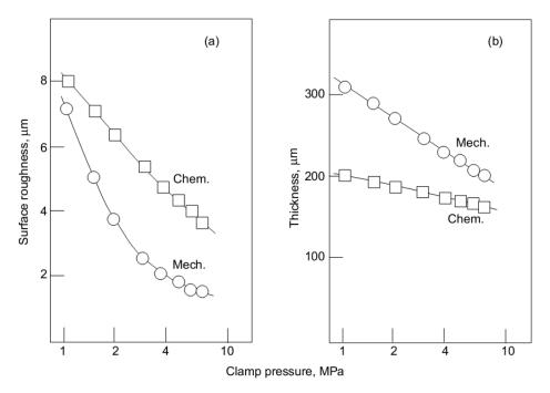
Figure 8. Surface roughness (a) and thickness (b) are depended on logarithmical scale of clamp pressure. [2]
