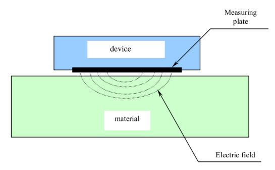
Figure 33. Dielectric principle of AP500 – M.
