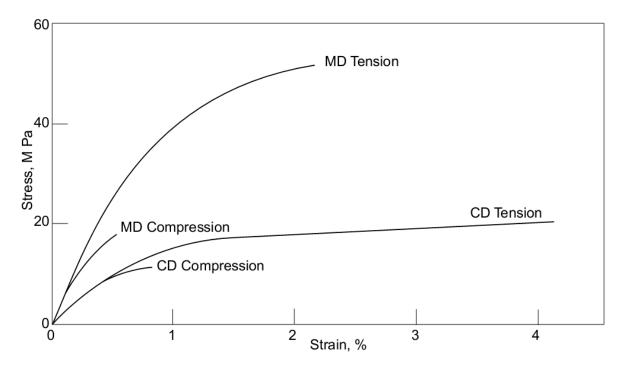
Figure 9. Stress-strain curve of a paperboard in tension and in compression. [2]
