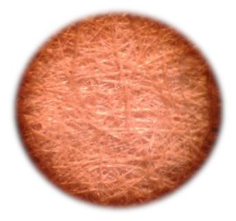
Figure 1. Virgin pulp on the microscope view.
