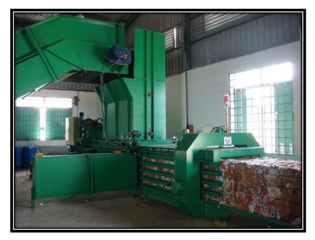
Figure 24. Horizontal waste paper baling press - Techgene Machinery Co., Ltd.
