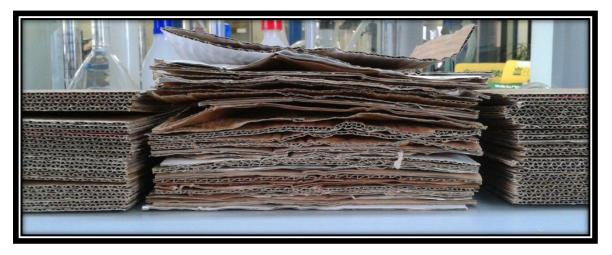
Figure 46. Sheet board samples – recovered board in the middle and virgin board
