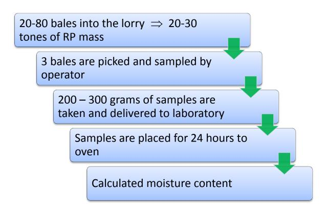
Figure 23. Approach of the oven-dried technique.
