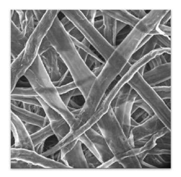
Figure 7. Scanning electron microscope image of a paper surface (KCL).
