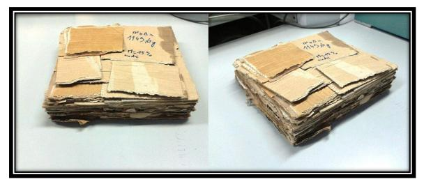
Figure 50. Recovered bale model 1.05 without residues.
