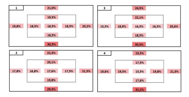
Figure 27. Moisture profile of "wet" bale (1.05), ref. No. 96105.
