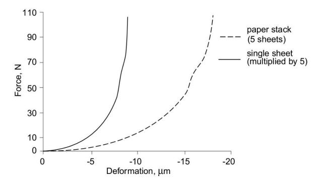
Figure 10. The out-of-plane stress-strain curve of a press-dried paper in compression. [2]
