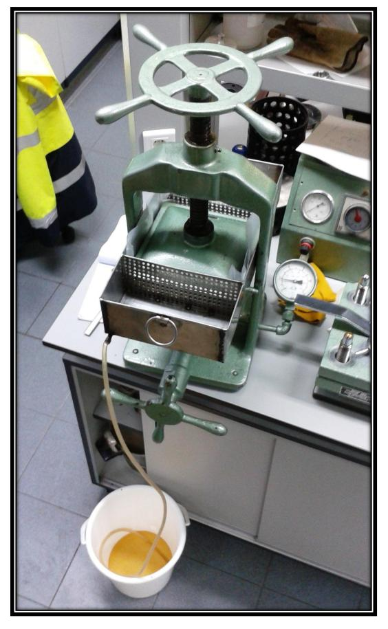
Figure 42. Hand - press apparatus with inserted metal container.
