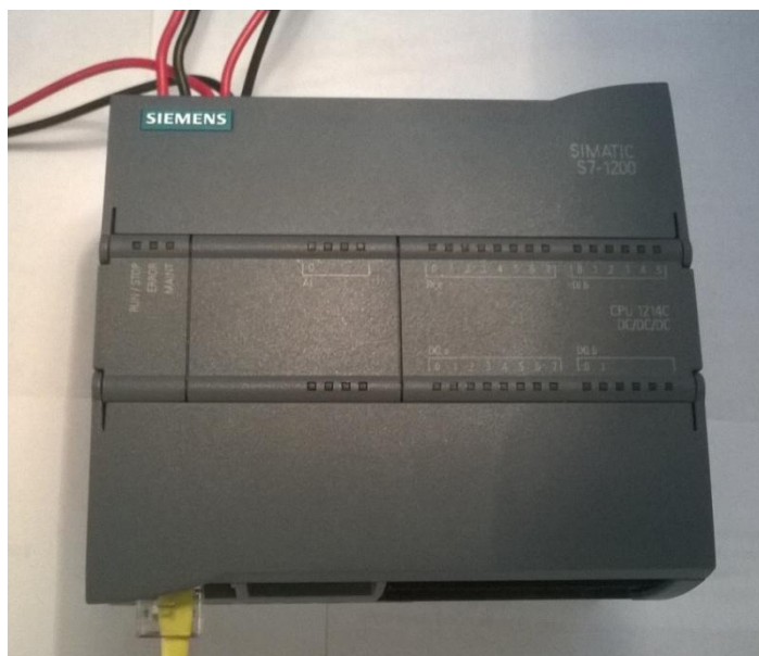
Obr. 12: CPU 1214C DC/DC/DC s kartou SB 1231 RTD
