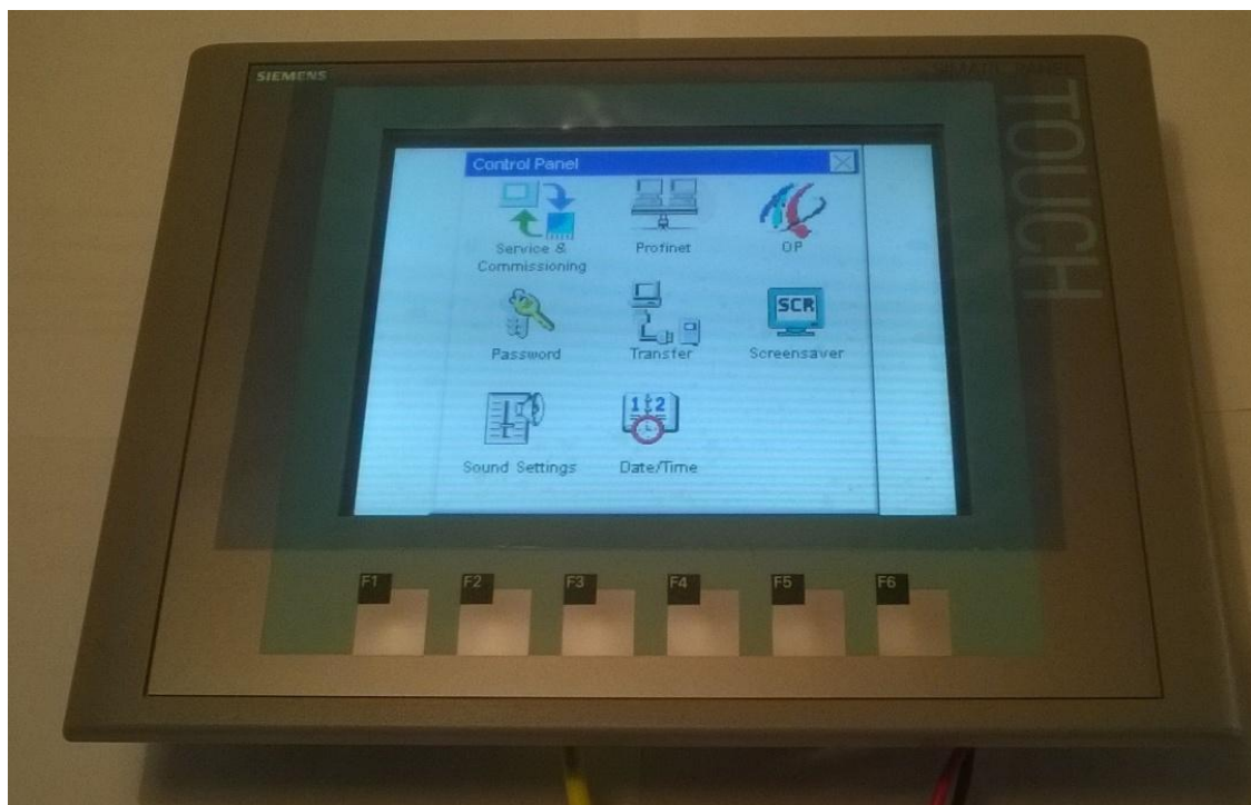
Obr. 16: HMI KTP600 Basic color PN
