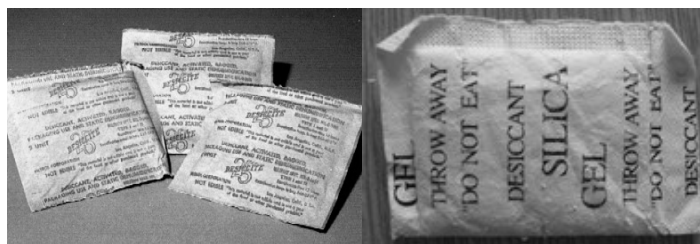
Fig. 5.2 – Examples of sacheted desiccants
