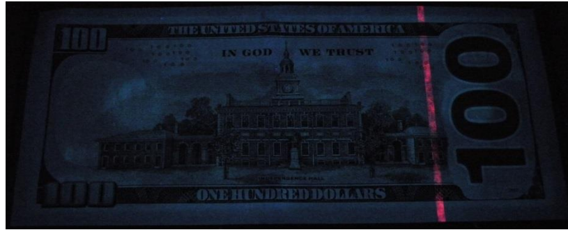
Fig. 133: 100 USD irradiated by 254 nm (front and back side)
