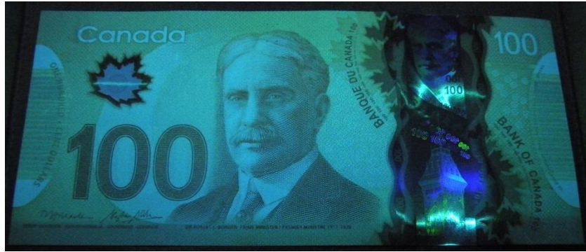
Fig. 172: 100 CAD irradiated by 366 nm
