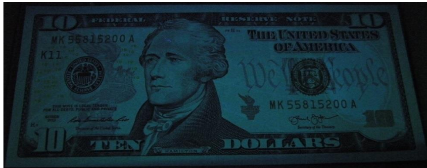
Fig. 116: 10 USD irradiated by 366 nm
