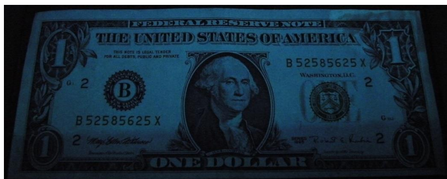
Fig. 103: 1 USD 1995/ 2013 irradiated by 254 nm
