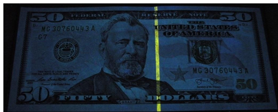
Fig. 127: 50 USD irradiated by 254 nm
