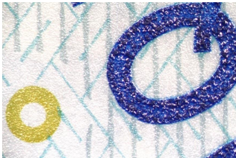
Fig. 155: 5 CAD (2013) feature against copying and raised ink
