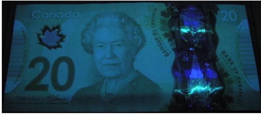
Fig. 164: 20 CAD irradiated by 366 nm
