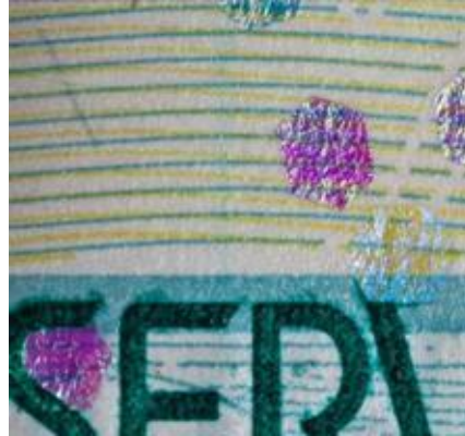
Fig. 36: Hexahedron planchettes with iridescent coating [11]
