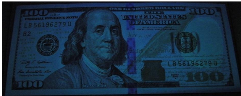
Fig. 133: 100 USD irradiated by 254 nm (front and back side)
