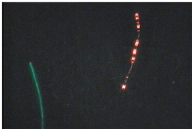
Fig. 4: Luminescence of security fiber [7]
