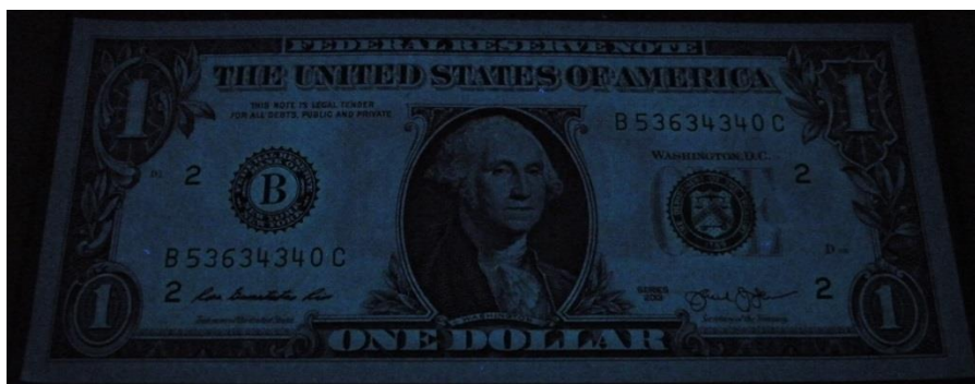
Fig. 103: 1 USD 1995/ 2013 irradiated by 254 nm
