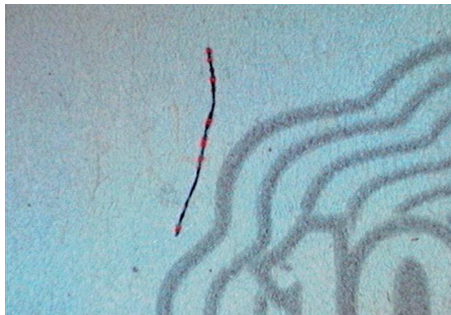
Fig. 3: Security fiber within paper structure [7]
