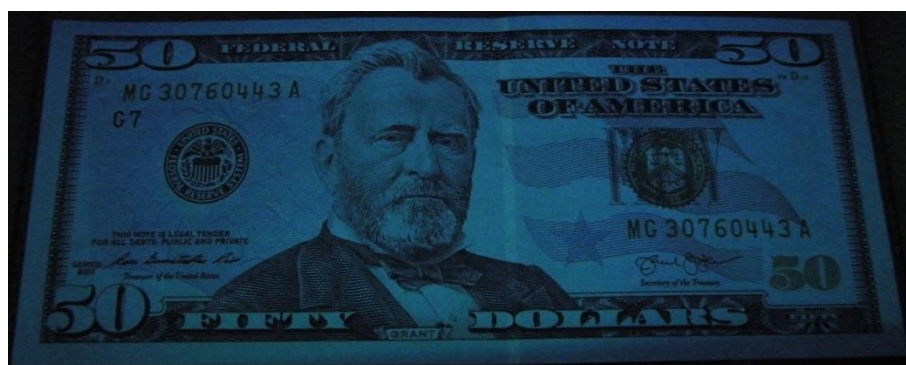
Fig. 128: 50 USD irradiated by 366 nm
