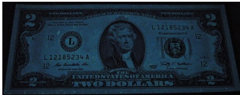
Fig. 107: 2 USD irradiated by 254 nm
