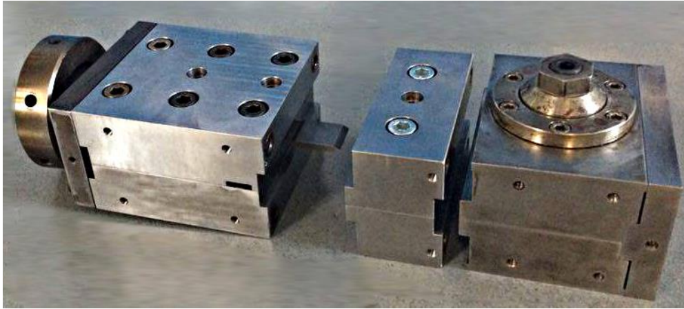
Figure 523: Constructed extrusion die without heaters
