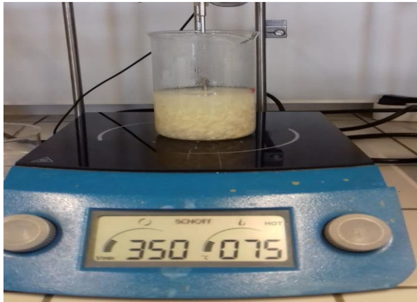
Figure 9: Extraction gelatine from pure collagen at 75 °C
