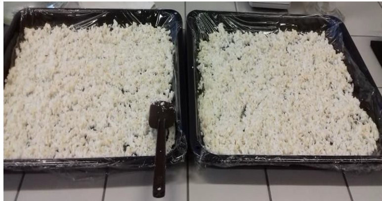
Figure 7: Evaporating solvent of collagen tissue
