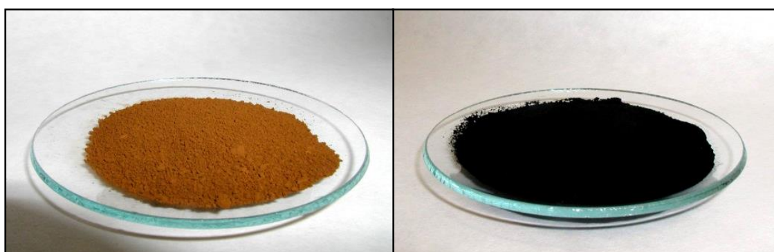
Fig. 34: The sample of surface unmodified pigment (left) and surface modified pigment of \text{ZnFe}_2\text{O}_4 using PANI. (Images were taken by Department of Paints and Organic Coatings, University of Pardubice)
