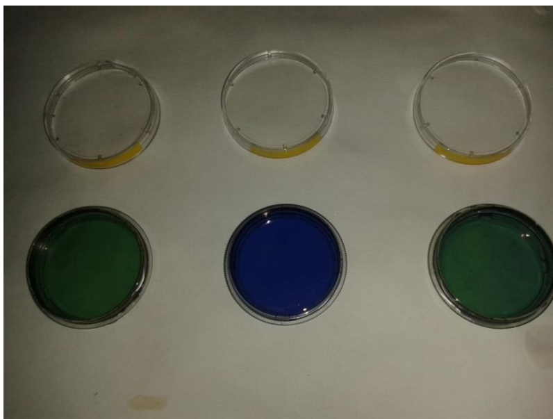
Fig. 14: PANI films prepared at the laboratory of the Centre of Polymer Systems by Nikola Mikušová. From left to right – green PANI-S, blue PANI-B and green PANI-S doped by PAMPSA.
