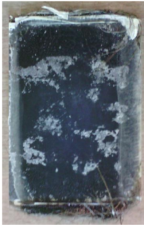
Figure 3.2: The produced BFRP composite plate. The compression machine pushed the excessive resin in the edges of the mold, contributing towards so as the composite structure to achieve high \Phi_f . Moreover, some small white pieces on the surface of the composite plate are just cook paper from the mold.
