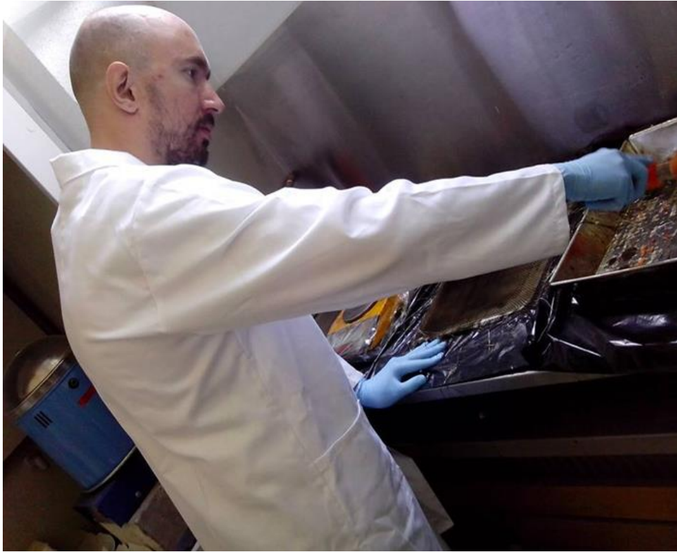
Figure 3.1: Preparation of the BFRP composites by the hand lay-up compression molding combined method
