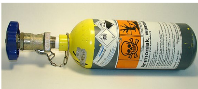
Figure 111: A small compressed gas cylinder with pure ammonia. [Source: Fig-111]
