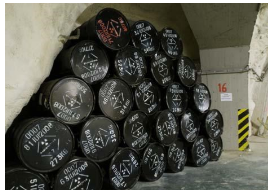
Figure 76: Disposal drums in the Richard radioactive waste repository. [Source: Fig-76]
