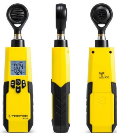
Photo 144: An apparatus for measuring formaldehyde in the atmosphere. [Source: Pho-144]
