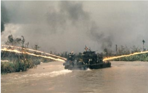
Photo 29: „Zippo” boat equipped with a flamethrower could fire compressed napalm up to 200 yards. [Source: Pho-29]
