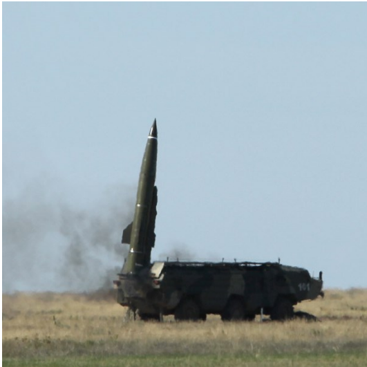
Photo 63: The 9M79 TOCHKA missile on the 9P129 missile launcher. [Source: Pho-63]
