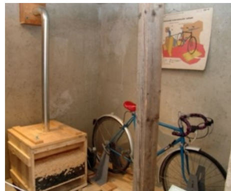
Figure 49: Example of an improvised shelter with air filtering equipment. [Source: Fig-49]
