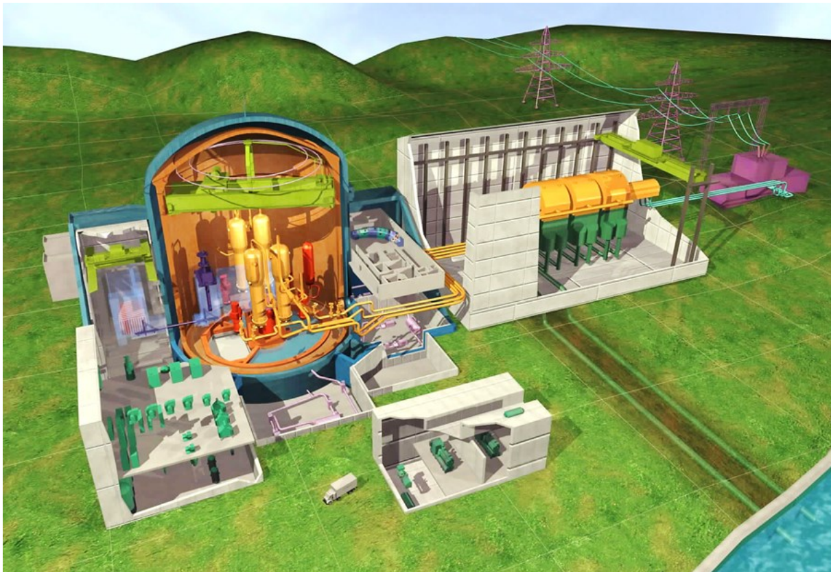
Figure 61: A virtual model of the section view through the unit with the EPR™ reactor. [Source: Fig-61]
