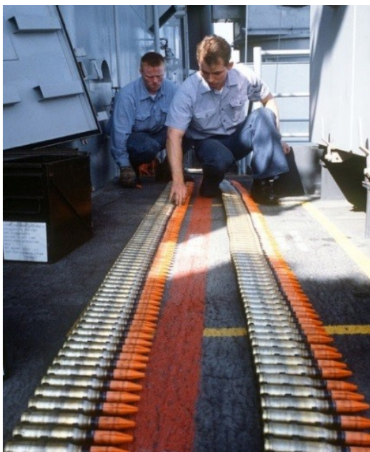
Photo 67: The belts of Mark 149 Mod 2 with 20mm DU ammunition on the battleship (USS Missouri). [Source: Pho-67]
