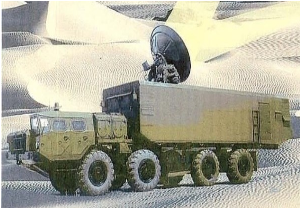
Figure 26: The Russian MMPS Ranets-E High Power Microwave (HPM) weapon system on the MZKT-7930 chassis. [Source: Fig-26]
