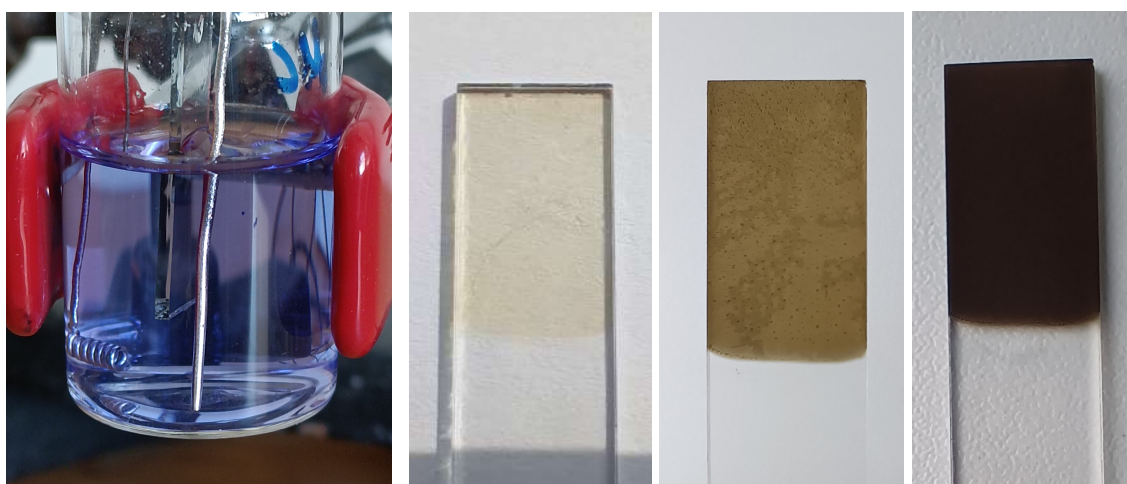
Figure 8.3 Electrochemically prepared PAZ: (left) the standard three-electrode cell with coiled Pt counter electrode, ITO glass working electrode, and Ag reference electrode; (right) films on ITO glass prepared from azulene concentrations 5 \times 10^{-4} , 1 \times 10^{-3} , and 5 \times 10^{-3} mol/dm 3 respectively. (Figure made by the author of this thesis).
