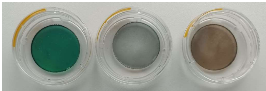
Figure 8.1 Conductive polymer films: (left) PANI, (middle) PPy, (right) PAz films on TCDs all prepared by in situ chemical polymerization oxidized with APS. (Figure made by the author of this thesis).
