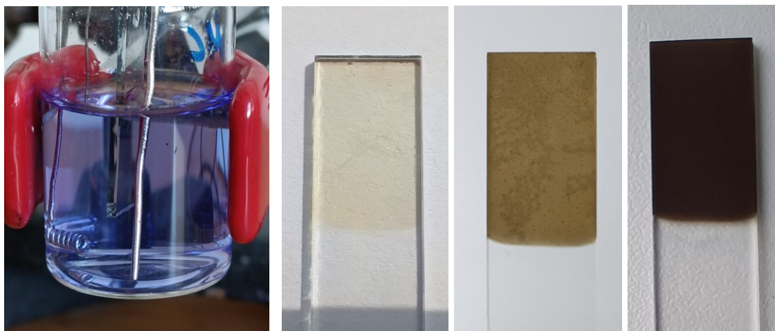
Figure 8.2 Electrochemically prepared PAz: (left) the standard three-electrode cell with coiled Pt counter electrode, ITO glass working electrode, and Ag reference electrode; (right) films on ITO glass prepared from azulene concentrations 5 \times 10^{-4} , 1 \times 10^{-3} , and 5 \times 10^{-3} mol/dm 3 respectively. (Figure made by the author of this thesis).
