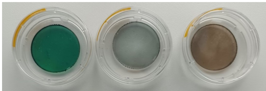
Figure 2.1 Conductive polymer films: (left) PANI, (middle) PPy, (right) PAz films on TCDs all prepared by in situ chemical polymerization oxidized with APS. (Figure made by the author of this thesis).
