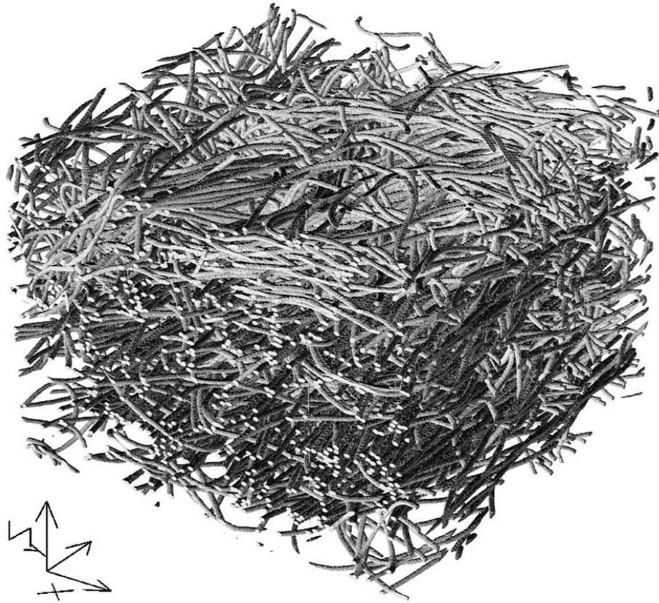
Figure 13: 3-D reconstructed DVI image from a nonwoven (800 x 800 x 600 voxels, with resolution 1.77 \mu\text{m}/\text{pixel} ) [85].
