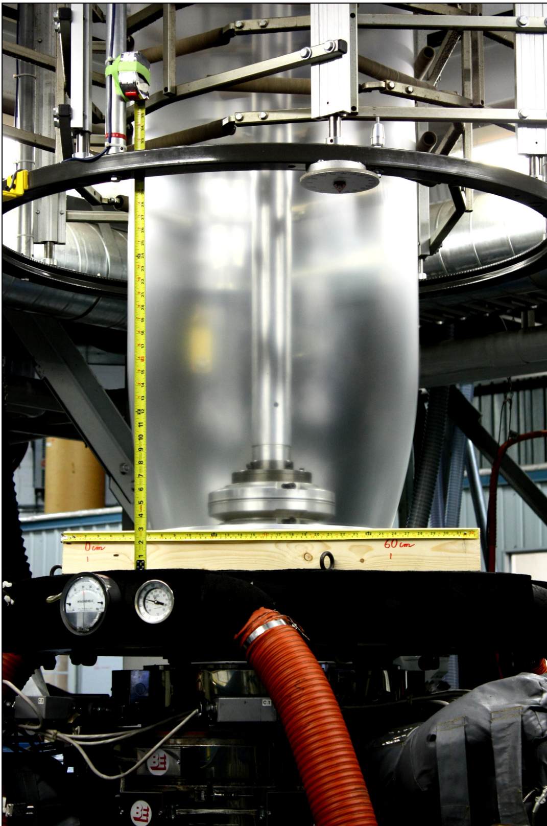
Figure 4. Detail view of the 9-layer film formation at Brampton Engineering multi-layer die exit region including the scale for precise bubble shape determination by using digital image analysis.
