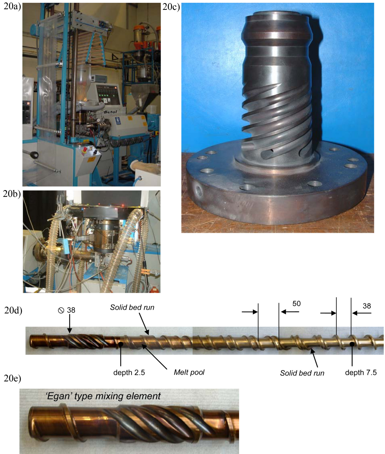
Figure 20. Film blowing experimental set-up. 20a) General view of the experimental film blowing line; 20b) Closer view of the film blowing die; 20c) Used spiral mandrel; 20d) DSBMT barrier screw with a 24:1 L/D and barrier flighted with spiral Maddox mixer; 20e) Detail picture of the Maddox mixer (egan type).
