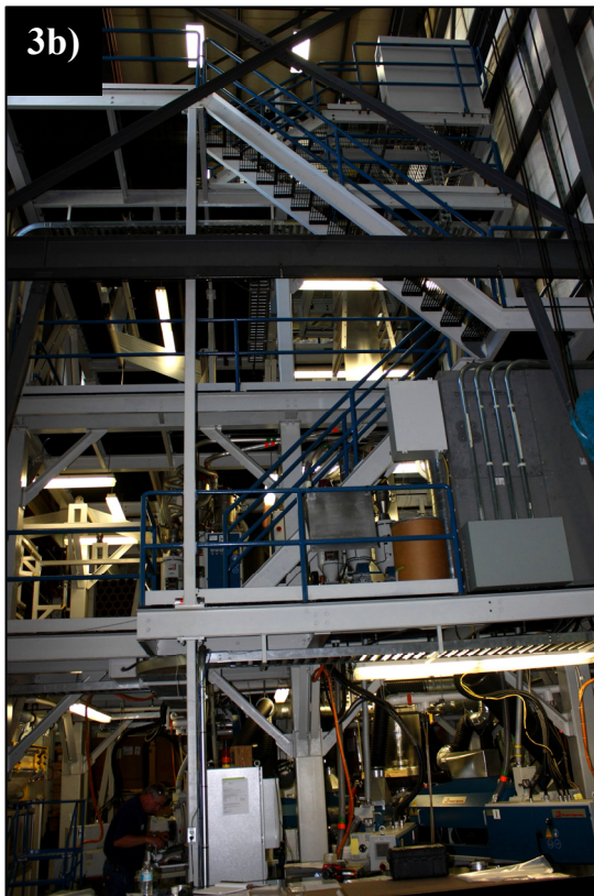
Figure 3. Brampton Engineering 9-layer air cooled blown film line.
