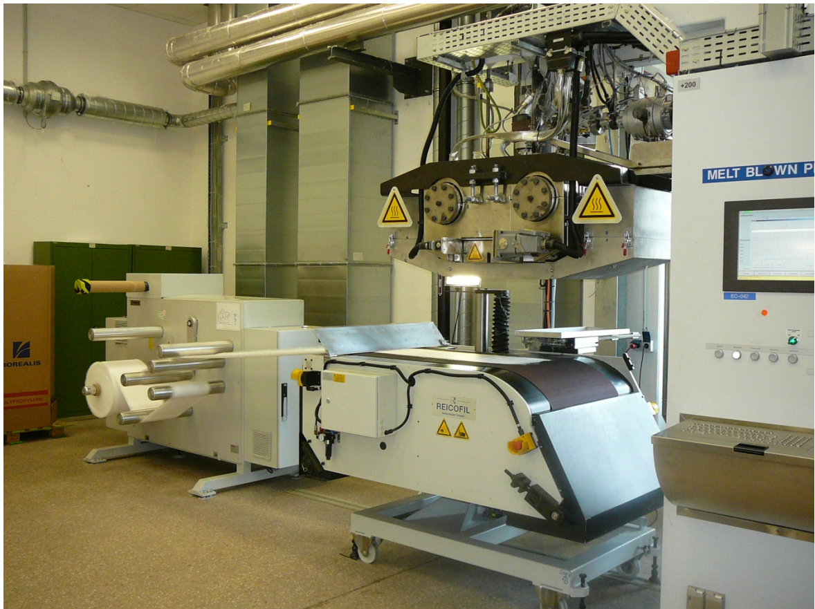
Fig. 47. Melt blown pilot plant line.
