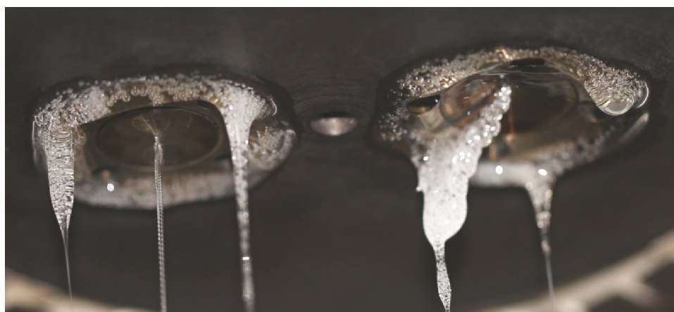
Fig. 56. Unwanted polymer melt leakage flow at the long die (left) and orifice die (right).
