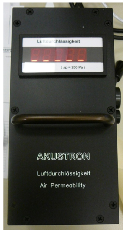
Fig. 55. Visualization of the AKUSTRON air permeability tester.
