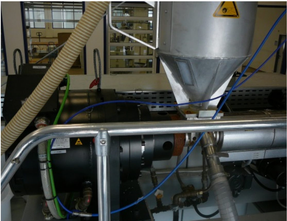
Fig. 48. Melt blown extruder. 48a, Control unit. 48b) detail view of the feeding part including the hopper. 48c) Detail view of the extruder heating belts.
