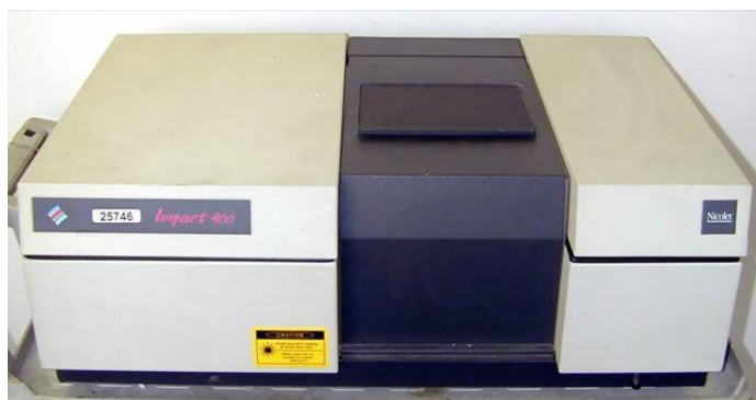
Obr. 27. Spectrometeres Nicolet Impact 400. [43]
