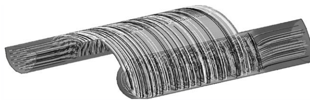
FIG. 12. Pathlines used for average stress calculation – mixer A.
