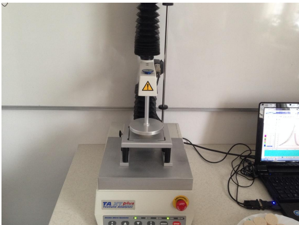
Obr. 6: Texturometr TA.XT Plus
