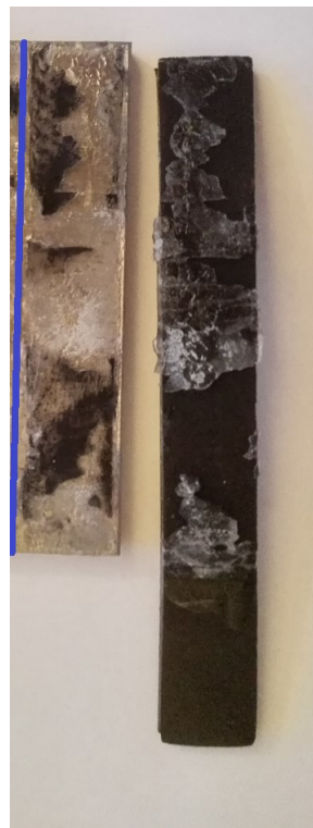
Figure 21 – Combined fracture (treated, tempered both, LQG)
