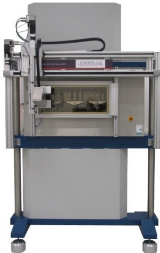
Figure 28 – Photo of Tear and Fatigue Analyzer – the version of 3 electro drives
