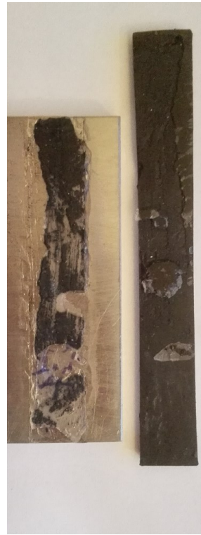
Figure 20 – Combined fracture (treated, tempered rubber, HQG)
