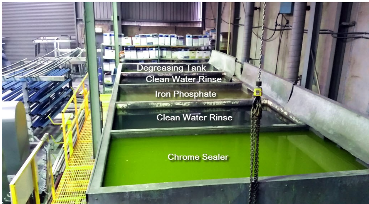
Figure 3 – Phosphate coating setup [9]
