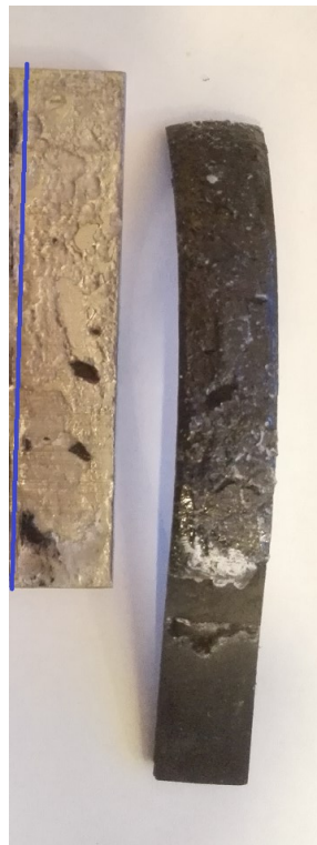
Figure 22 – Cohesive fracture of glue (treated, tempered both, LQG)
