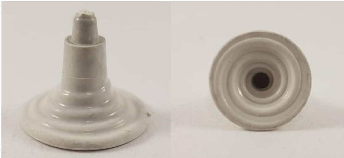
Figure 33 – Design of tested Al 2 O 3 PIM part
