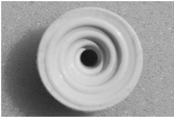
Fig. 1 Design of tested aluminium oxide PIM part
