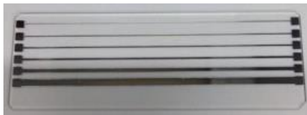
Figure 17 – Ink-jet printed silver lines array on microscopic glass slide. Width of lines is pixelated as 1, 3, 5, 10, 20 and 40 pixels. Length of 71 mm was kept constant.
