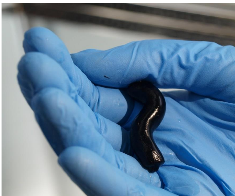
Figure 5. Polyaniline cryogel mimicking the properties of native tissue. Source: Cell biology laboratories, Centre of polymer systems, Tomas Bata University in Zlin.
