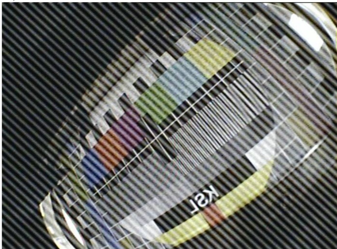
Fig. 4. Camera Streaming in the GTEM Chamber with a Level of 30 V/m.
