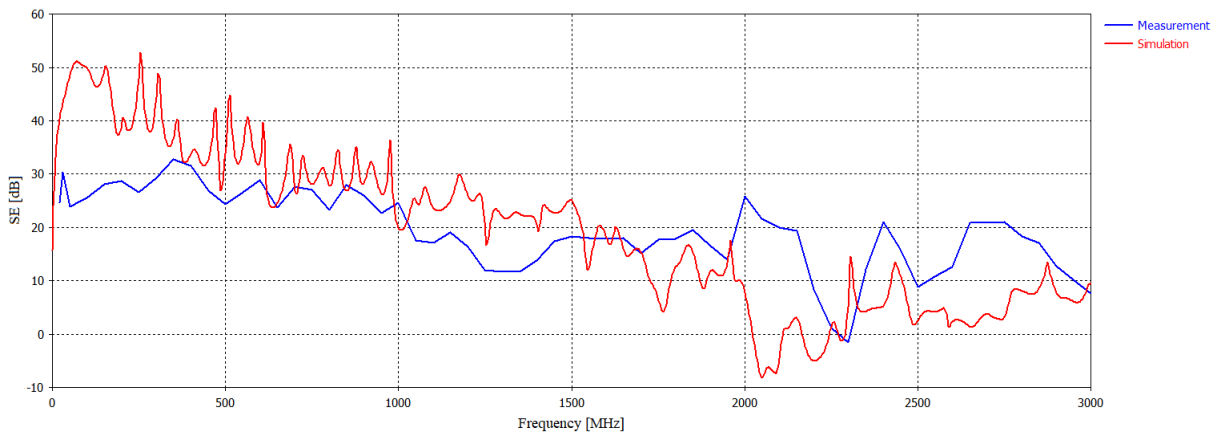
Fig. 7. Shielding Effectiveness Comparison of Measurement and Simulation – Shielding enclosure B.
